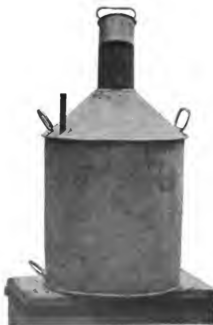
SPECIAL CAN FOR FILLING FUEL TANK OF RACING CAR QUICKLY.
